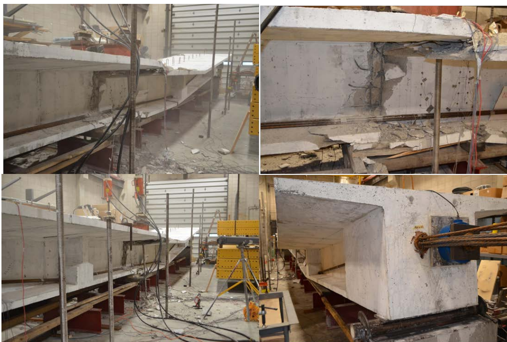
Figure 3.22 – Girder UNB2 after Failure (Sritharan et. al., 2018)
