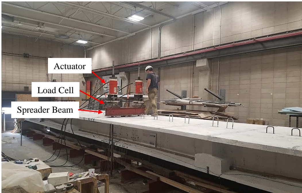
Figure 3.14 – Test Setup for Segmental Girders (Sritharan et. al., 2018)
