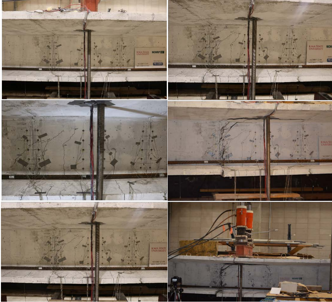
Figure 3.21 – Progression of Crack Formation beside the Segment Interface in UNB2 (Sriharan et. al., 2018)
