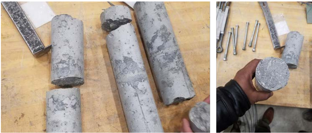
Figure 3.7 – Failure of Cylinders Connected with Epoxy from Tensile Test (Sritharan et. al., 2018)
