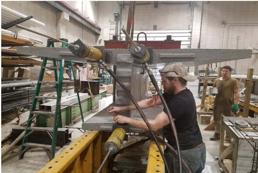
Figure 3.8 – Application of Temporary Post-tensioning Force (Sritharan et. al., 2018)
