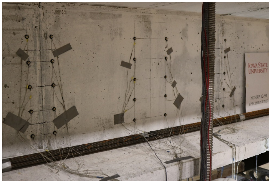
Figure 3.13 – Optoktrak 3D LED layout for Girder UNB2 (Sritharan et. al., 2018)
